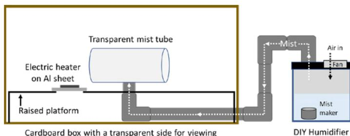
An example of a clear, simple scheme for a rather complex experimental setup to show convection currents, which would be very difficult to illustrate clearly with a photograph.
