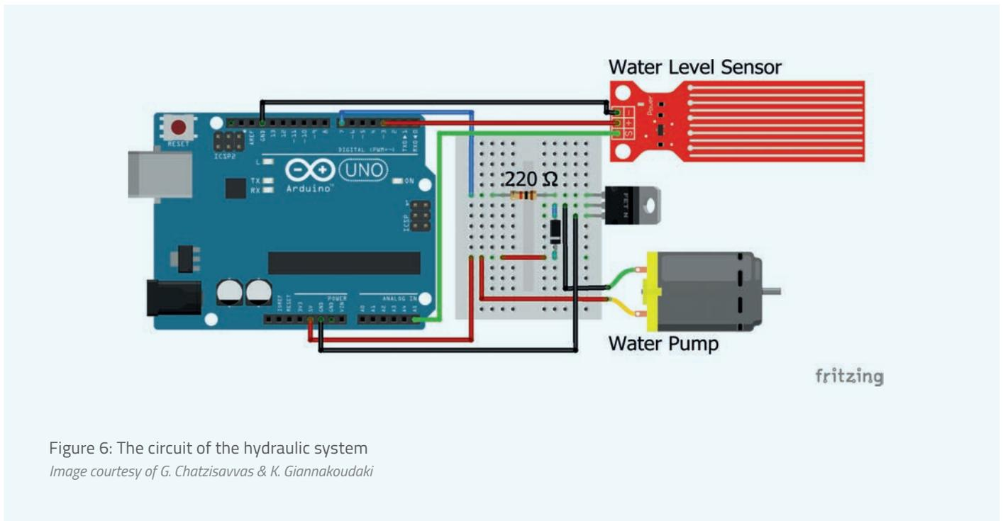
Figure 6: The circuit of the hydraulic system
