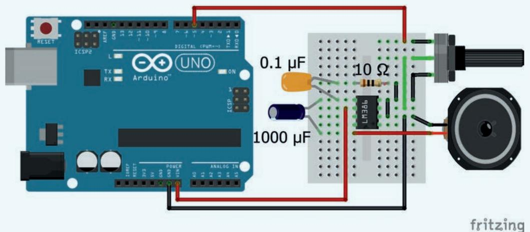
Figure 4: The circuit of the sound system
