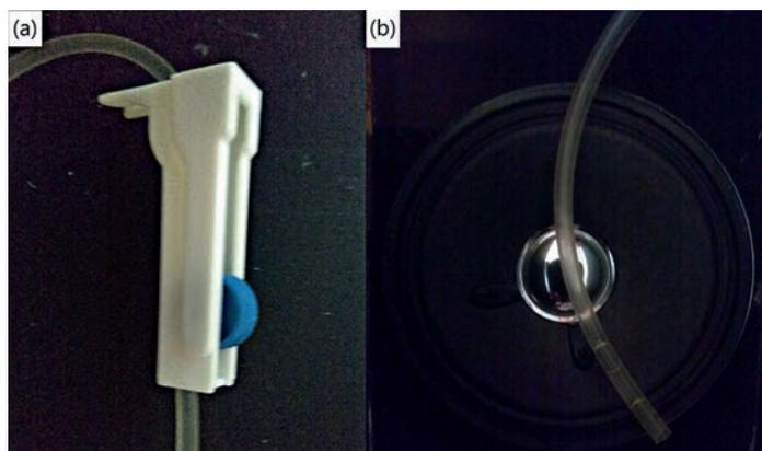
Figure 2: The water flow controller (a) and the speaker (b)
