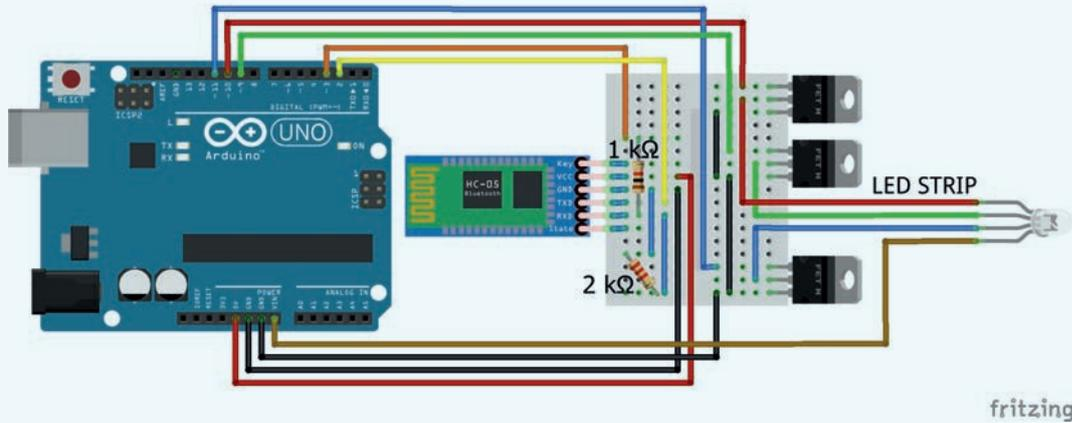
Figure 3: The circuit of the stroboscopic system
