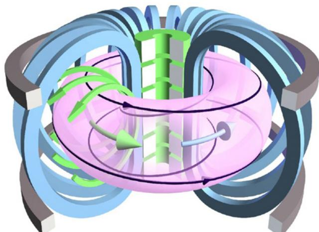
Schematic of a tokamak – the magnetic coils (shown in blue and grey) are used to control the fusion plasma (in pink)
